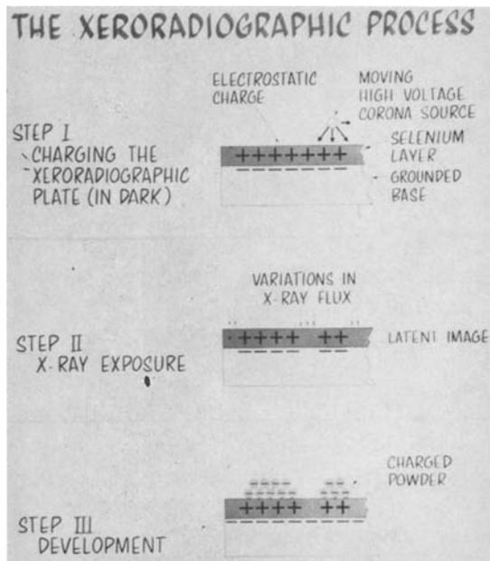
Fig. 1. Xerography is possible because selenium is a photoconductor. An electrostatic charge placed on its surface will remain in an absence of radiant energy. X rays make the selenium conductive perpendicularly. After exposure there is a residual charge pattern which may be made visible by "developing" with a negatively charged, pigment-containing powder.
