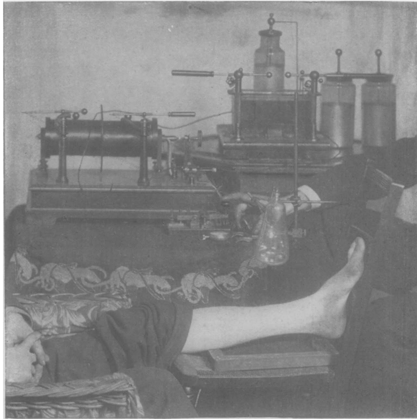
PHOTOGRAPH OF APPARATUS AND METHOD EMPLOYED FOR OBTAINING A SKIAGRAM. IN THIS CASE THE LEG.
