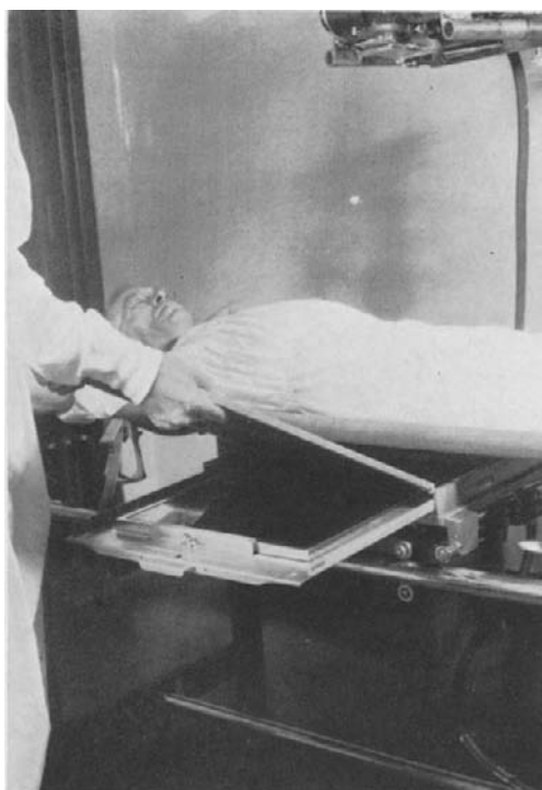
Fig. 6. The portable grid unit mounted on the horizontal carriage, in position for roentgenography. Note that vertical adjustment has been made so that the grid is at the level of the litter sag. The wafer grid itself is being lifted out from its housing, as is possible when it is needed for use in the ward. Note the cassette beneath the grid and its accommodation in a standard cassette tray.
